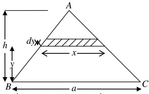
$$I_{BC} = \int_0^h (x\rho dy)(y^2) = \frac{a}{h} \rho \int_0^h (h-y)(y^2) dy = \frac{1}{6} M h^2$$
