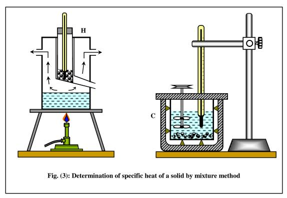
The solid, in the form of a small pieces, is weighted and suspended inside the heater by a thread passing through the cork. Steam is passed
