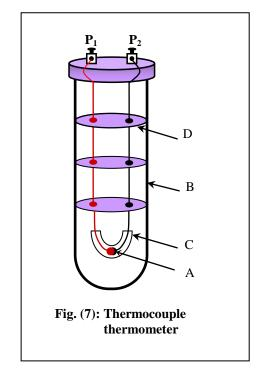
These two wires are then passed through mica disks D closely fitted in the tube B and attached to terminals  $P_1$ ,  $P_2$  fixed on the cap closing the mouth of tube. To these terminals long wire of the same metals are also
