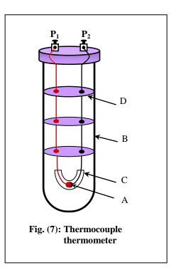
These two wires are then passed through mica disks D closely fitted in the tube B and attached to terminals  $P_1$ ,  $P_2$  fixed on the cap closing the mouth of tube. To these terminals long wire of the same metals are also connected to form a cold junction being immersed in melting ice at  $0^{\circ}$ C at a fairly distance place from hot junction.
