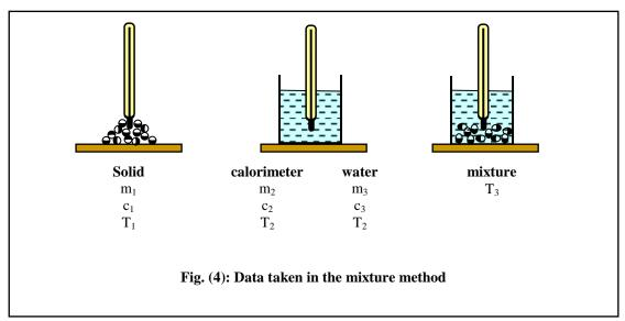
Suppose  $c_1$  is the specific heat of a given solid.  $m_1$  grams of the solid at  $T_1^{o}C$  is added to  $m_3$  of water at  $T_2^{o}C$  in a calorimeter whose mass is  $m_2$  and its specific heat is  $c_2$ . Let  $T_3^{o}C$  be the final temperature of the mixture, see Fig. (4). By equating the heat lost by the solid  $Q_s$  to the heat gained by the calorimeter and water  $(Q_c + Q_w)$  we get
