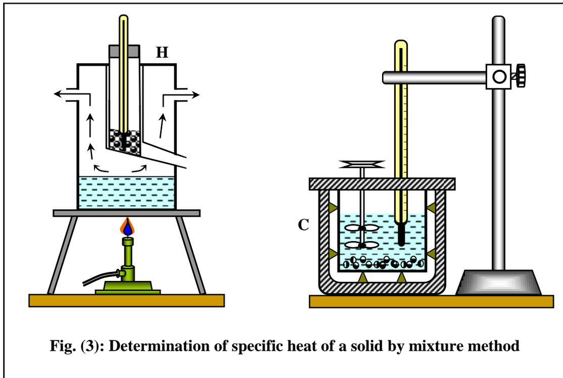
The solid, in the form of a small pieces, is weighted and suspended inside the heater by a thread passing through the cork. Steam is passed through the heater from a boiler, so that the solid may be heated without actual contact with steam or water. While the solid is heated, the empty
