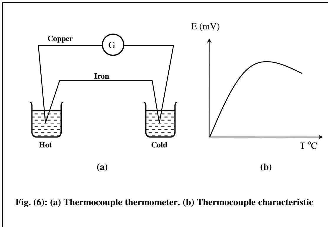
Fig. (6): (a) Thermocouple thermometer. (b) Thermocouple characteristic
